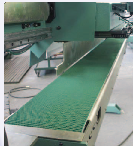
Motorised belt for multiple area unloading
